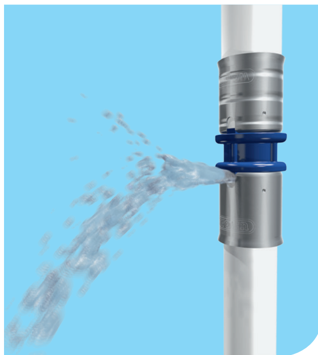
Figure 4: Safety through clever technology: the Defined Leak Function in the pressure test reveals unpressed fitting connections
